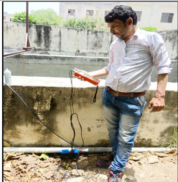
Measurement at STP outlet
