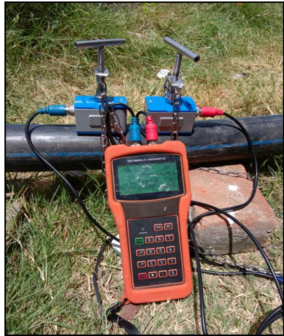
ultrasonic flow Meter installation at university tank
